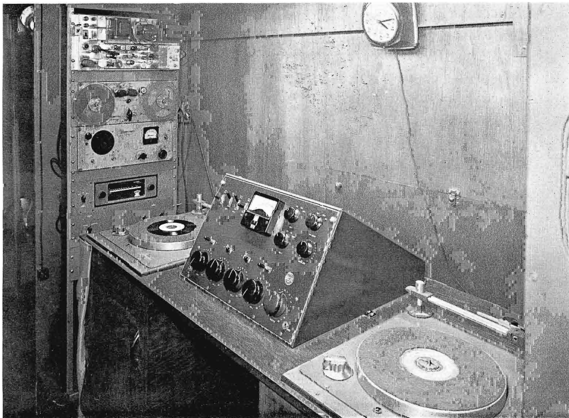
FIG. 8. Complete equipment in WERE mobile unit includes a tape recorder. The equipments external to the console are rack-mounted. All switching is readily available to the operator. On location, it is only necessary to plug in the microphones.
