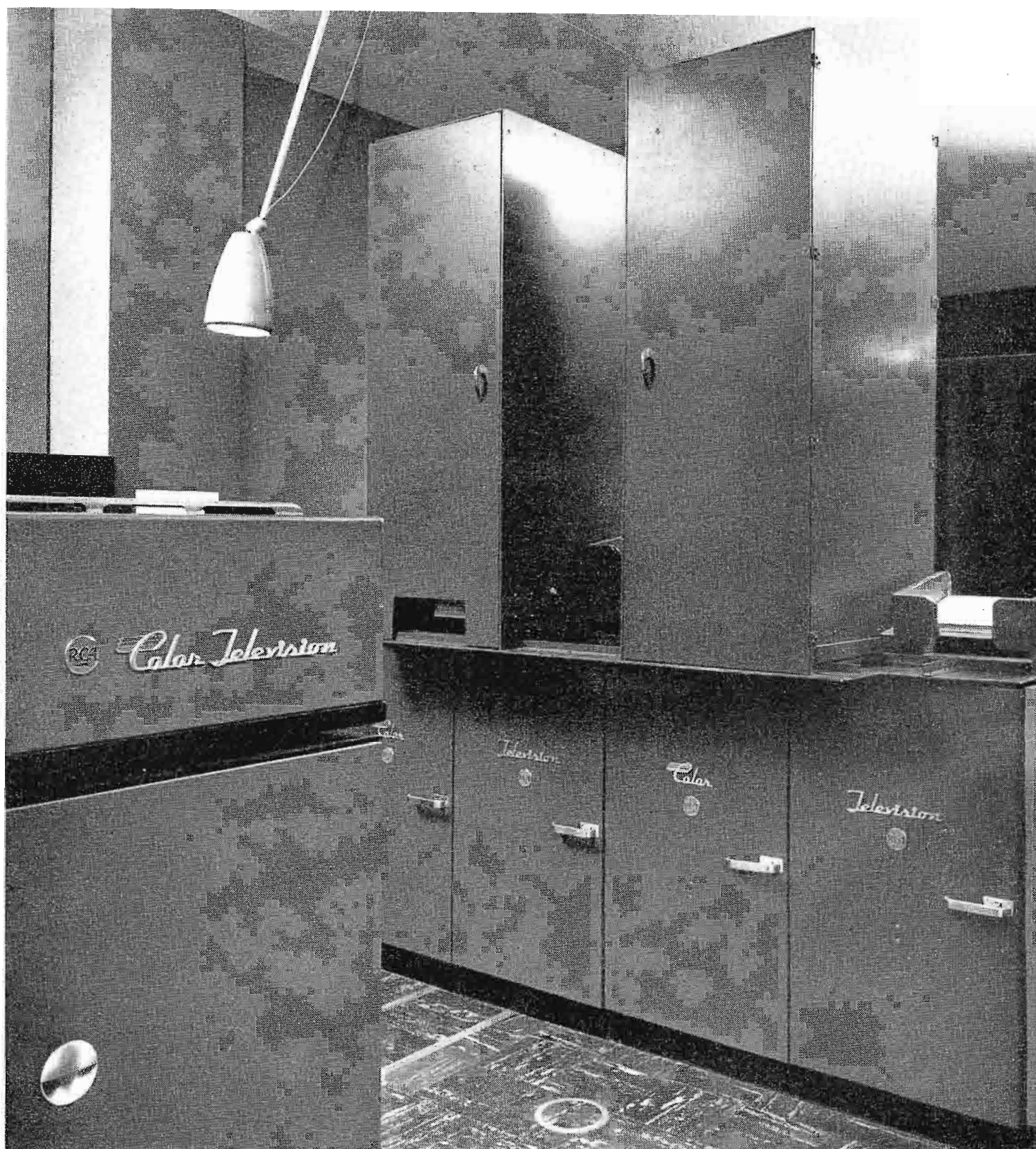
FIG. 32. Another view of WBTV's film room showing the two Chromascan units used for projecting color opaques.
