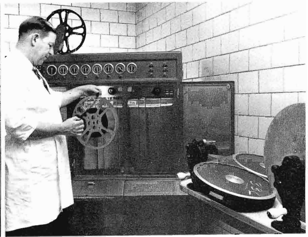
FIG. 37. WBTV uses this Filmatic to get pictures on the air minutes after the undeveloped film is brought in by the station's camera crews.
