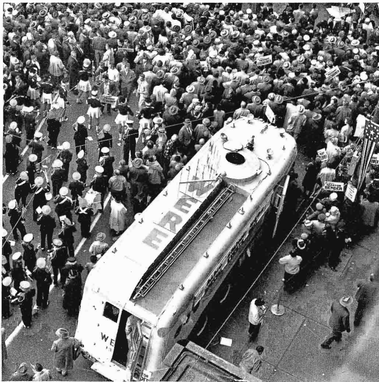
FIG. 4A. WERE mobile unit in use at the 1956 presidential political campaign meetings. Note that turret is in "recessed" position.
