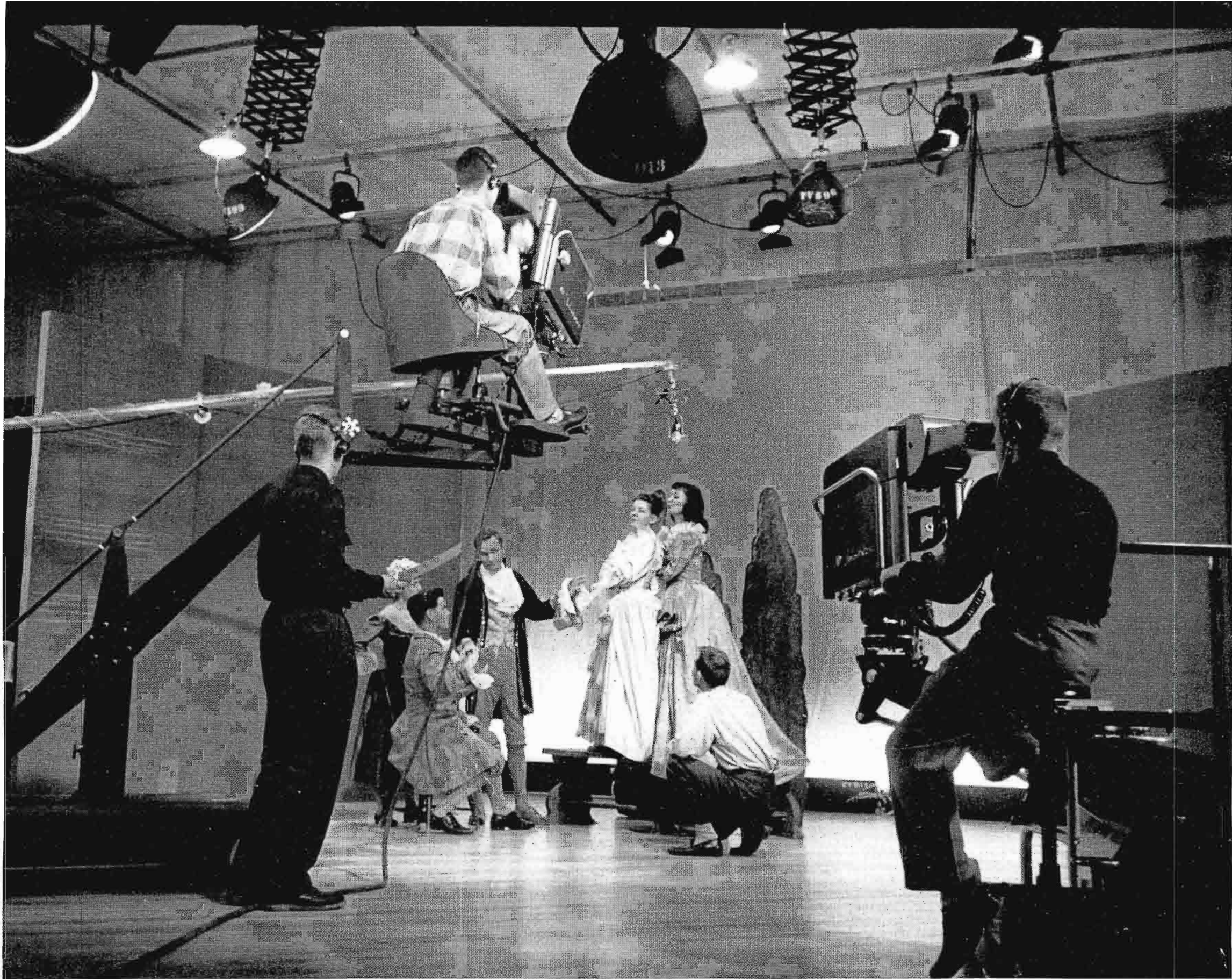
FIG. 1. TV education courses. Workshop for TV courses is the main studio professionally equipped with RCA TK-11 Studio Cameras, microphone and lighting equipment.
