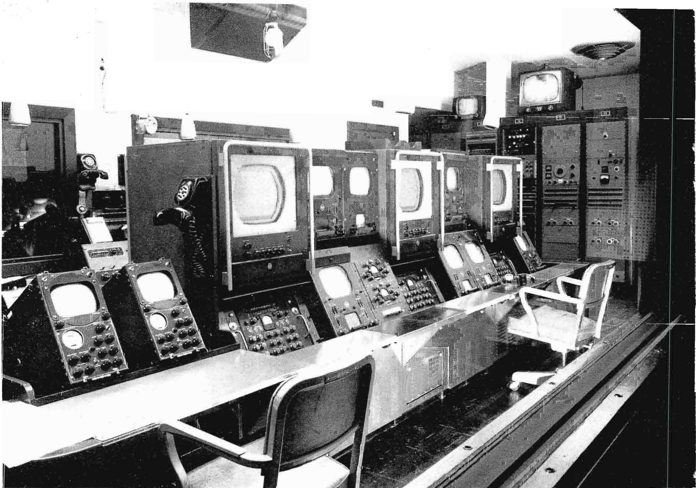
FIG. 18. WBTV's video control console as seen through the window from the \alpha -m control room (see floor plan, Fig. 6). Camera control for four monochrome studio cameras, one color studio camera, two 3-V color film cameras and two color Chromascan units are incorporated in this console. Monitors are provided for both monochrome and color operation. Location of the various units in this console is shown in Fig. 19. Video operators at this position make all necessary camera adjustments. Camera switching is done by the director in the studio control booth.
