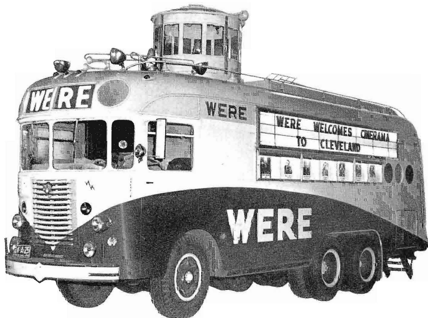
FIG. 4. Mobile studio-on-wheels proves to be the ultimate for doing traveling disc-jockey shows. This WERE unit is equipped to operate independently of outside facilities. The turret on top is used by the announcer at outdoor public events. It is raised and lowered by hydraulic operation, off the engine.
