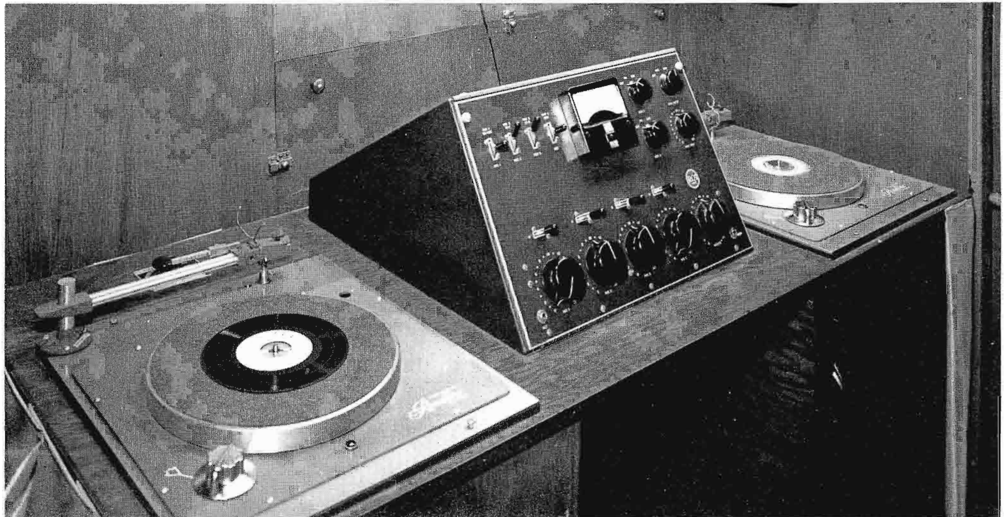
FIG. 6. Control console inside WERE mobile unit. Three-speed turntables are used. An RCA Type BC-5A Audio-Consolette is employed. The complete control console can be removed as a unit for use in semipermanent remotes.
